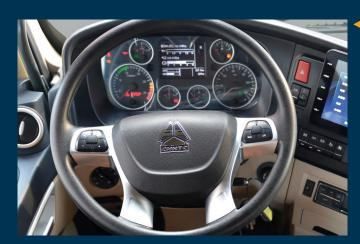
**Ergonomics-oriented design:** instrument switches and door switches are laid out reasonably, while electric doors and windows, electrical rear mirrors are easy to operate; steering wheel is pneumatically controlled so that it could be adjusted by height and angle, contributing to high degree of ergonomics.
