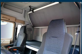
Super-wide sleeper: flat-roofed M cab with 525mm wide sleeper and flat-roofed W cab with 749mm wide sleeper provide more comfortable rest space for driver and pessengers.
